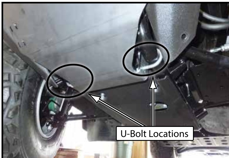
"Figure 3" U-Bolt Install
