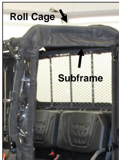
6. Wrap the subframe textile around the subframe and roll cage. Attach using velcro on the fabric.
