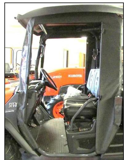
7. Adjust the fit of the textiles so they are taugth with minimal wrinkles.
