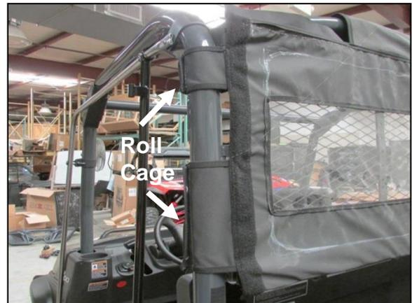
1. Attach the back panel by strapping it to the rear vertical roll cage bars on both sides.
