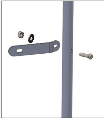
1. Attach the Bent Subframe Bracket (M) with a M6 x 30mm socket head bolt, nut and washer.
