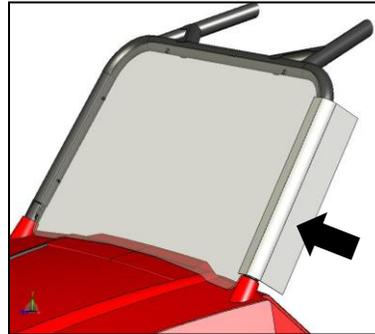
This method is best for full 1pc windshields where user doesn't plan on switching it out after install as Velcro will adhere directly to windshield edge surface. It increases seal slightly but installation is a bit trickier. The surface to adhere the Velcro must be cleaned well, but alcohol should not be applied to acrylic or polycarbonate.
