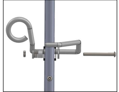
2. Assemble the door handle in the order shown above with the ¼ - 20 x 2.5" Bolt and nut. Place the metal washers and plastic spacers between door and inside door handle. You may have to adjust the number of washers and spacers so the door closes against the subframe securely.
