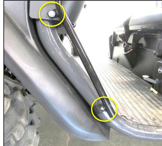
3 & 4. Loosely bolt the front of the subframe to the front of the vehicle using the M8x20mm socket head bolt. Bolt the bottom with M6 x 30mm socket head bolt, nut and washer.
