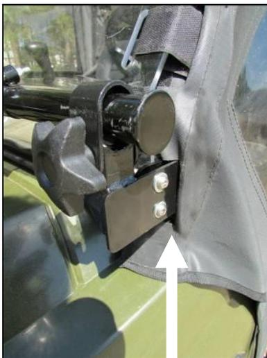
The side panel textile needs to be cut to accommodate the hood rack roll cage clamp / brackets.
