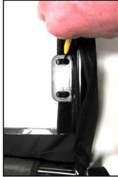
Locate plate behind inside Velcro flap & mark to punch holes in fabric.
