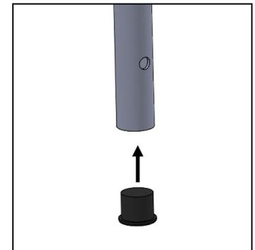
4. Push End Plug (J) into end of the tubes.
