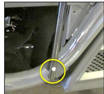
7. Loosely attach the bottom of the rear subframe to the clamp near the vents of the vehicle using a M6 x 35mm bolt, nut and washer.
