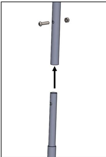
2. Attach the Upper Subframe (A) to the Lower Front Subframe (B) with a M6 x 25mm socket head bolt and nut.
