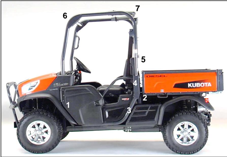
**In the next few steps, you will be installing self adhesive velcro on the vehicle in the positions shown. Clean all surfaces with rubbing alcohol before installing Velcro Strips**
