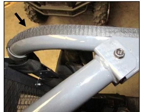
**7. Adhere Velcro straps to upper rear corner the roll cage as shown. They should line up with the Velcro on the fabric.**
