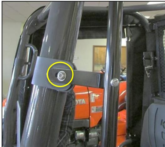
2. Loosely attach the front of the subframe to the clamp on the front of the vehicle using a M6 x 20mm bolt, nut and 2 washers.
