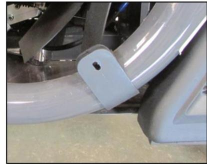
3. Place a clamp in the bottom rear corner of the roll cage in the location shown.
