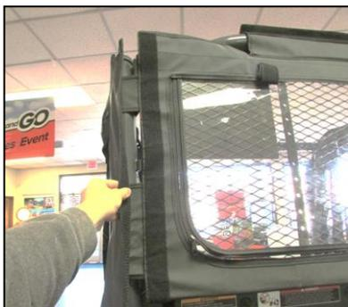
5. Attach the subframe textile to the velcro strip on the back panel.
