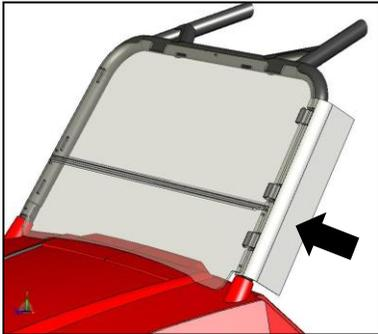
This is preferred method. Best used for 2pc., folding, & ½ windshields. Side Panel Velcro's directly to Roll Bar. Notches are cut into side panel to accommodate mounting system. Minimizes interferences with 2pc. & folding windshield functions.
