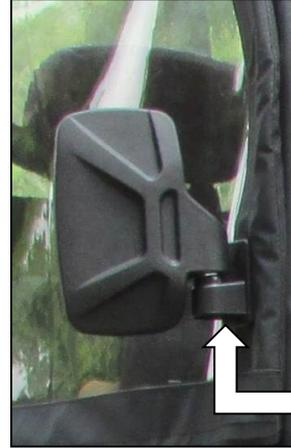
Install mirror with supplied hardware. Adjust position as required.
