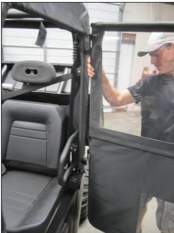
5. Mount the doors by guiding the pins in the back of the door frame onto the hinge barrels along the Door Hinge Subframe.
