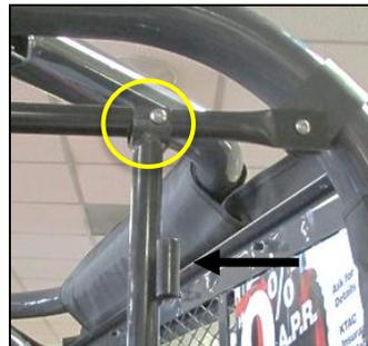
6. Attach the rear subframe to the front subframe with a M6 x 30mm socket head bolt and nut. The door hinges should be closer to the back of the vehicle.
