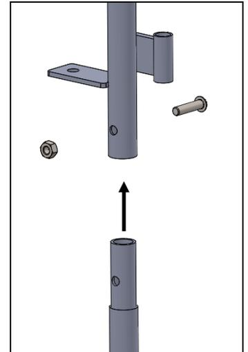
3. Attach the Door Hinge Subframe (C) to the Lower Rear Subframe (D) with a M6 x 25mm socket head bolt and nut. The hinge will be on the back side of the tube.
