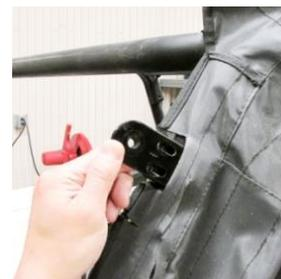
8. Install light bar bracket & bar
