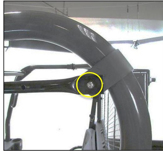
1. Loosely attach the front subframe to the clamp on the rear of the vehicle using a M6 x 20mm bolt, nut and washer. The washer should be between the plastic clamp and the nut.
