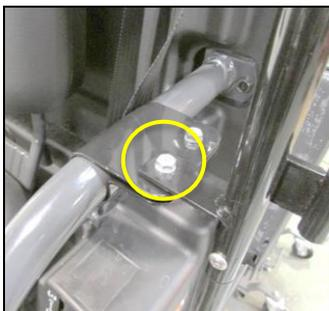
5. Set the rear subframe on TOP of the door hinge clamp. Loosely bolt with M6 x 20mm bolt, a nut and two washers.
