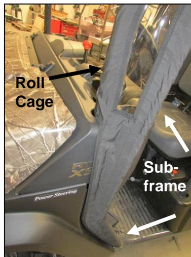
3. Wrap the subframe textile around the front subframe and roll cage and attach using velcro on the fabric.
