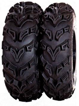
Most V-shaped lug patterns usually slide a lot under braking. Not these. When you grab a handful of brake lever, they dig into the dirt hard. You can probably give most of the credit to the steps on the backside of the lugs. They have multiple biting surfaces to help dig in. The fact that the tires weigh slightly less than similar-sized mud tires doesn't hurt, either.
