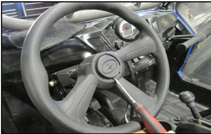
Then remove the center nut with a 24mm socket. To remove the wheel you will need to hit it slightly on the backside to break it free. If it does not come off then you might need to use a wheel puller to remove it.
