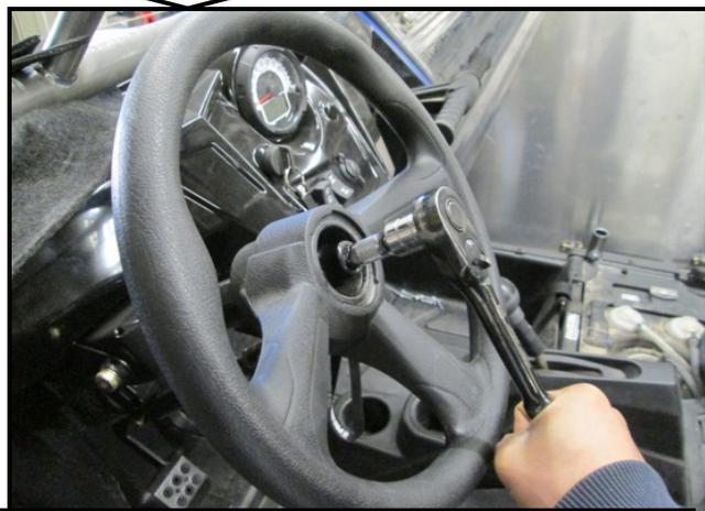
Fully remove the OEM steering wheel and replace it with the steering wheel hub adaptor. The hubs fits several models so the shaft might differ slightly from picture below.
