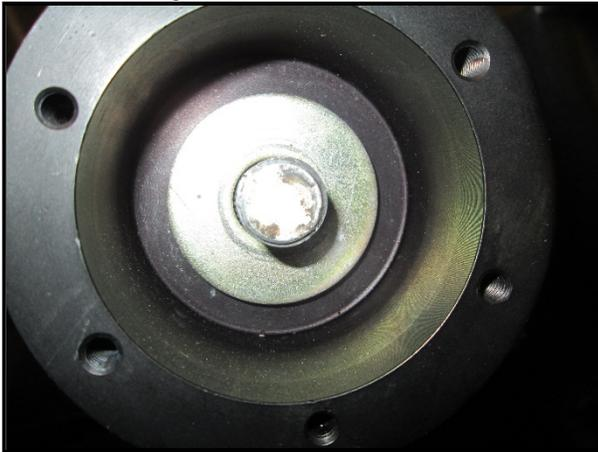
After tightening the large factory nut, grab the hub like shown and shake up and down, and left and right, to make sure there is no movement. If the hub has movement repeat the steps, or call Pro Armor customer service for help.
