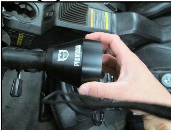
Re-install the factory nut on top of the 2 provided washers and tighten the nut to the vehicles manufacturers recommended torque specifications. Before final tightening, make sure the hub is aligned so the steering wheel is straight when driving straight.
