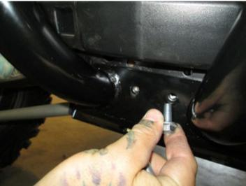
• Fasten the lower portion of the bumper to the car using the supplied lower mounting bracket assembly [ITEM 1] and M8 bolts [ITEM 2]. The lower mounting bracket assembly will go behind the mounting bracket on the chassis. Do not fully tighten.
