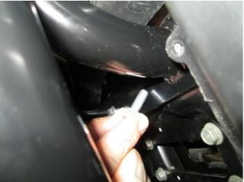
• Fasten the upper portion of the bumper to the car using the supplied M8 bolts [ITEM 2] and upper mount PEM nut plate assembly [ITEM 3]. The upper mount PEM nut plate assembly will go behind the mounting bracket on the chassis (or behind the adapter plate for 2014 model vehicle applications). Do not fully tighten.
