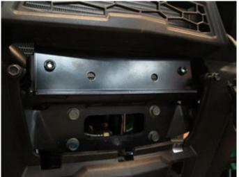
• If you are installing on a 2014 model vehicle, you will need to install the adapter plate [Item 4] using the supplied M8 bolts [Item 2] and M8 washers [Item 5]. Make sure the flanges on the plate face outward and the inner holes are offset towards the bottom when installed.
