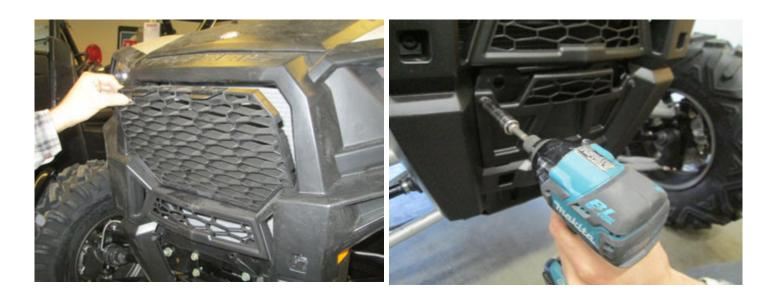
• Remove the stock plastic grill by pulling down on the upper tabs and pulling out. Then, remove the lower plastic guard by unfastening the (2) stock M6 screws.
