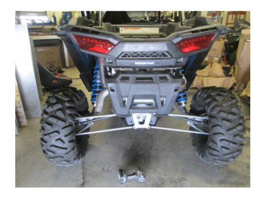
• Remove the 2 M6 bolts holding the muffler support bracket to the chassis, on each side of the vehicle.
