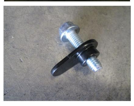
The supplied M10 bolts [Item 1] and winged nuts [Item 2] will be used to fasten the lower mounting brackets of the bumper to the chassis. The winged nut will allow you to tighten the M10 bolts without having to hold the nut on the other side, since space is very limited between the chassis mounting area and rear differential. Place the bumper onto the car and line up the mounting brackets to the chassis. You may need to work the lower
