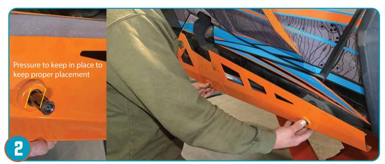
Once you have all (3) anchors in the chassis holes, maintain pressure and tighten down until snug. Do not stop tightening so anchor remains in place.
