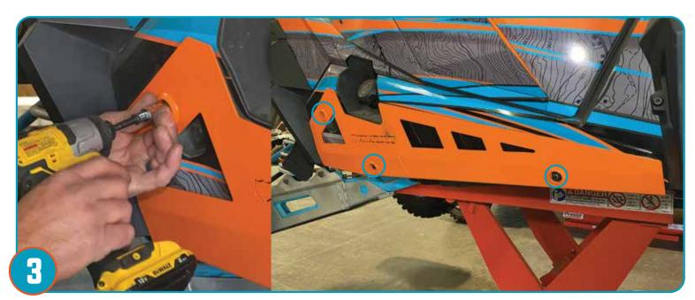
Keep the rock slider snug up against the plastic as you go around and evenly torque down the three anchors. DO NOT OVERTIGHTEN as you may shear the bolt in the expansion anchor.
