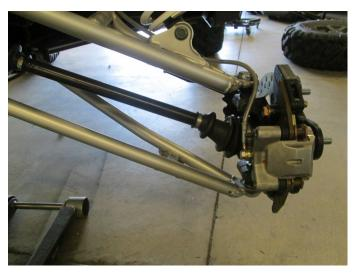
• Place a-arm guard on a-arm and loosely install mounting hardware as shown. Adjust a-arm guard to ensure best fitment. Then, tighten down all hardware.
