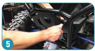
Position skid onto rear bumper mounted to vehicle and tighten claps to bumper securing skid to rear bumper.
