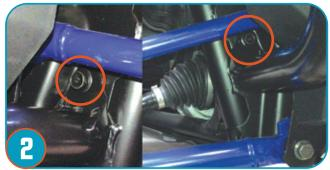
Insert lower bolts and nuts to both sides of bumper, securing bumper to frame.
