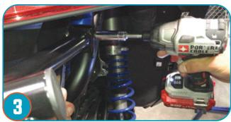
Tighten rear bumper upper and lower bolts firmly securing rear bumper to frame of the vehicle.
