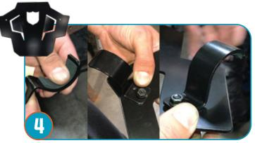
Apply provided rubber strips to skid plate clamps as shown. Using provided bolts and nuts, attachand hand tighten clamps to the Rear skid.
