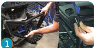
Align Bumper to rear of vehicle lining up bolt holes, inserting a bolt and nut to both sides to support and position bumper in place before tightening to factory specs.
