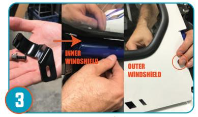
Using the provided (2) brackets/bolts, secure the lower windshield tightening the bracket, threading bolt from outer windshield through bolt hole and through bracket /nut on inside securing windhsield to cage. One Bracket per bottom of windshield.
