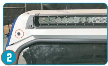
Tighten upper windshield with (2) provided bolts. One on each top corners as shown.
