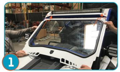
Place windshield on vehicle sliding the top of windshield under roof, lining up the bolt holes. The roof comes with rubber washers that are used in the same holes that the windshield mount. When installing the windshield. The frame of the windshield replaces the washers supplied with roof.
