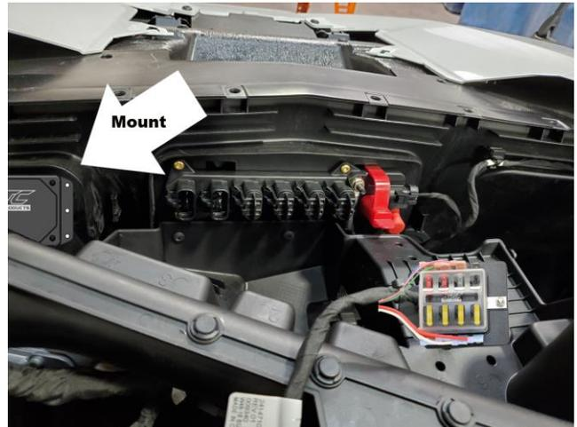
3. Mount the Fuse Box on the spot marked by the #2 Arrow. The reason for mounting it at this position is that you can get to the fuse box through the door on the dash without removing the dash cover.
