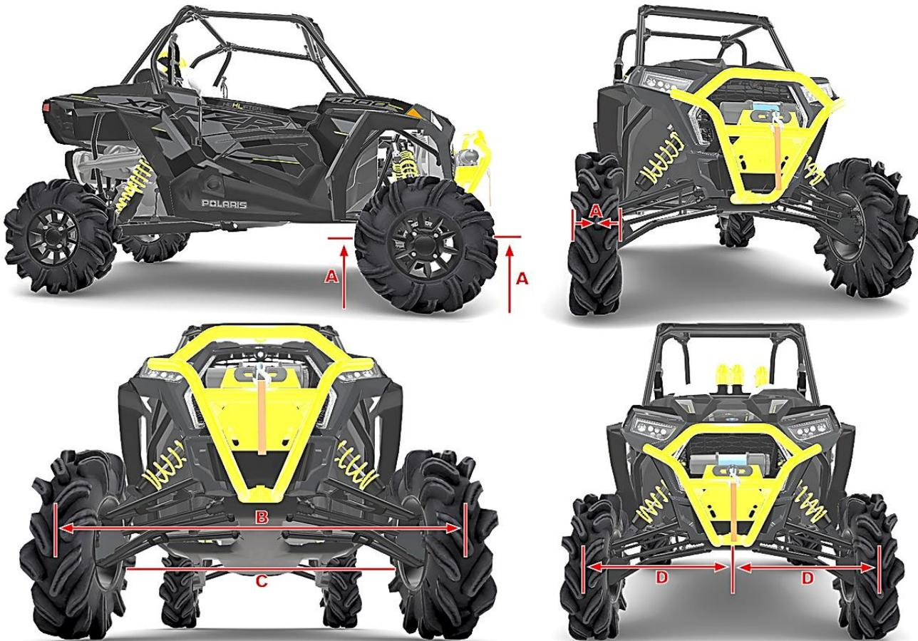
Place the machine on a smooth level surface and set the steering wheel in a 'straight ahead' position. Secure the steering wheel in this position.
