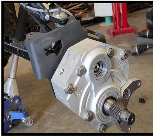
**Loosely fasten all (4) bolts with 1/2" flat washers and 1/2" lock nuts. Ensure parts fit correctly then torque.**
