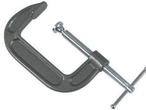
**If upper ball joint spins while installing, use a c-clamp to clamp the ball joint to the backing plate.**
