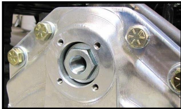
c. Align the portal box lid cap & gasket. Use the 1/4-20 x 3/4" screws and install to the box. (5/32) [8 ft lbs]
