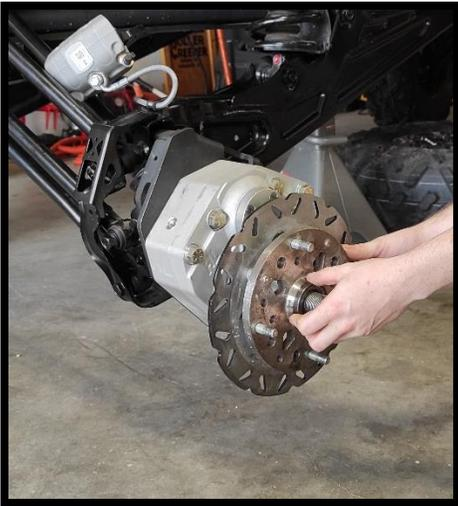
b. Slide on the supplied **30mm lock washer**, followed by the **30mm spindle castle nut**. (46mm) [Min 120 ft lbs] Tighten the castle nut further if needed to align grooves with holes in the spindle for the cotter pin. Install the supplied **cotter pin**. Both ends of the cotter pin must be folded.
