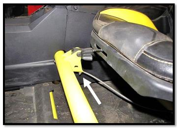
c. Drill out the rivets securing the factory p-clamps to the trailing arms.
