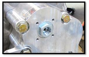
c. Align the portal box lid cap & gasket. Use the 1/4-20 x 3/4" screws and install to the box. (3/16) [8 ft lbs]
