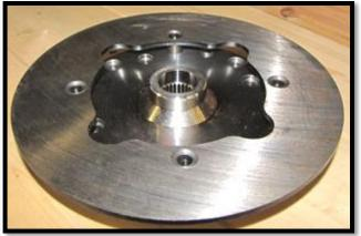
b. Apply **LOCTITE (RED)** to (4) **3/8-16 x 1" button head bolts**. Insert the screws through the rotor, the spacers, and then into the hub. Tighten and torque. (7/32) [45 ft lbs]
