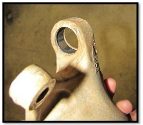
d. Inspect the radial joints for excessive wear or damage. If they show significant signs, they need to be replaced.
