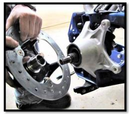
d. Remove the nuts that attach the rear knuckle to the radius bars. (15mm) Only pull the bolts out far enough so that the knuckle can be released. This way you don't have to disconnect the radius bars. Then remove the knuckle.
