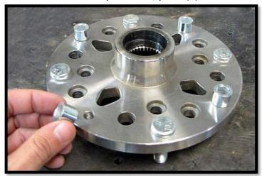
a. Locate a **brake rotor PGLC-ROTOR-2**. The side with the counter bores should be facing up. Place the rotor on to the hub and line the holes up with the tapped holes.
