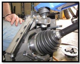
c. Position the lower ball joint into the lower ball joint mounting bracket on the backing plate.
