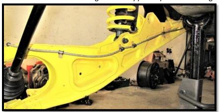
d. There's one rivet that isn't easily accessible. You can either remove the seats and drill through the plastic to remove them. Or what we recommend, you can simply cut the brake lines near the p-clamp (Have area prepared for brake fluid clean up). The factory lines and this p-clamp will not be re-used.
