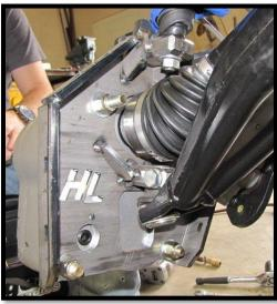
e. Install the tie rod end into the backing plate tie rod mount bracket. Fasten the tie rod end with the factory hardware. (18mm) [90 ft lbs]
