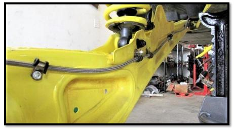
i. Fasten the new t-block to the factory location using the factory hardware. **Do not over-torque**. And then secure the brake lines to the seat frames using the factory nuts.
