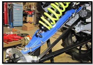
c. Disconnect the front factory t-block from the frame. (It's at the front of the firewall above power steering).
