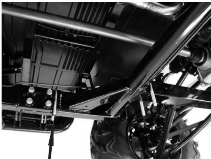
Rear U-Bolt position just in front of the four bolts holding the frame together
