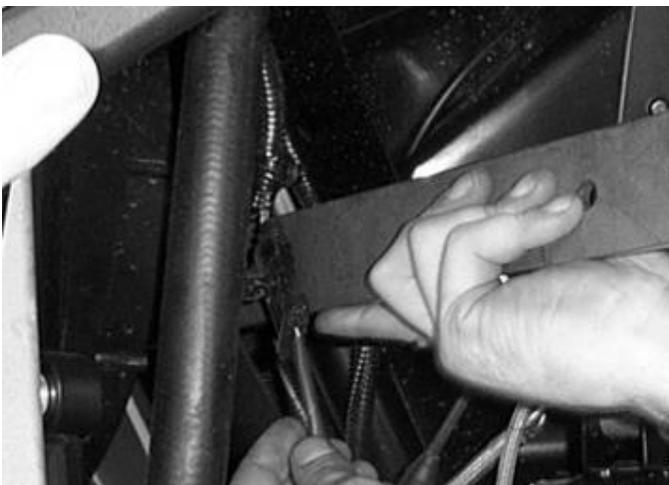
31. Depending on which side you are working on you will place either a left lift bracket or right lift bracket to the outside of the front shock mount. It needs to be on the side that faces the front of the UTV. Connect the bracket using two 10x65mm hex bolts and four 10mm flat washers. Insert the two bolts through the bracket, then place two washers on each bolt. Insert the bolts through the shock mount tabs.
