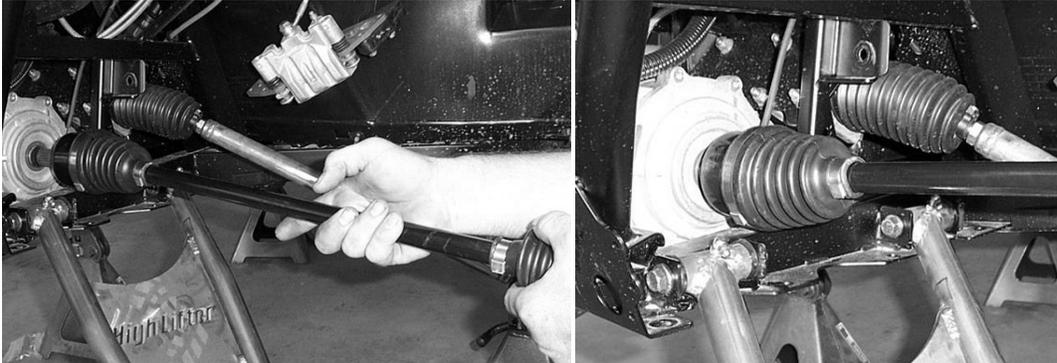
40. With the axles in place, slide the hub assembly over the axle and connect it to the lower control arm. Use the factory hardware.
