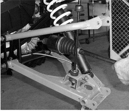
8. Remove the nuts that secure the sway bar to the sway bar rod. You will completely remove the sway bar, sway bar connecting brackets, and rods from the UTV. They are not used in conjunction with the big lift kit.
