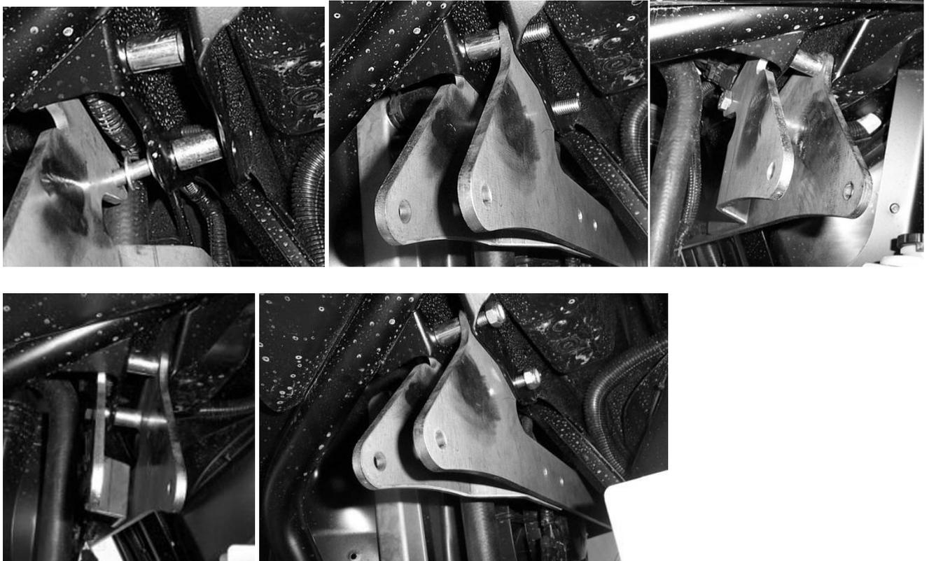
33. Use two 10mm x 35mm bolts to secure the short front lift brackets to the long front lift bracket.
