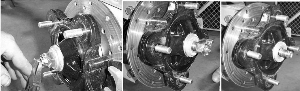
5. Remove the brake rotor assembly.
