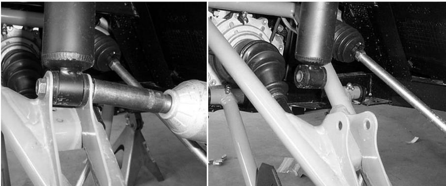
10. Unclip the brake lines from the control arms. Tie the calipers up out of the way.
