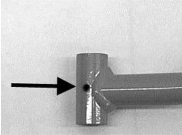
17. Once you have removed the stock bushings, sleeves, and ball joints from the factory arms install them into the new arms in the kit. If you place some grease on them it makes the installations easier.
