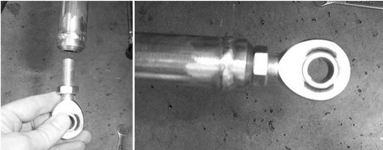
54. Once you have drilled the hole, use the  $\frac{1}{2}$  x 4-1/2" hex bolt and the two high alignment bushings, large cone and connect the heim joint to the knuckle.
