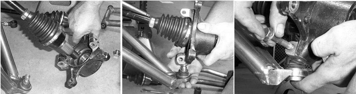
41. Next, connect the upper control arm to the frame and then to the hub assembly. Use the factory hardware.
