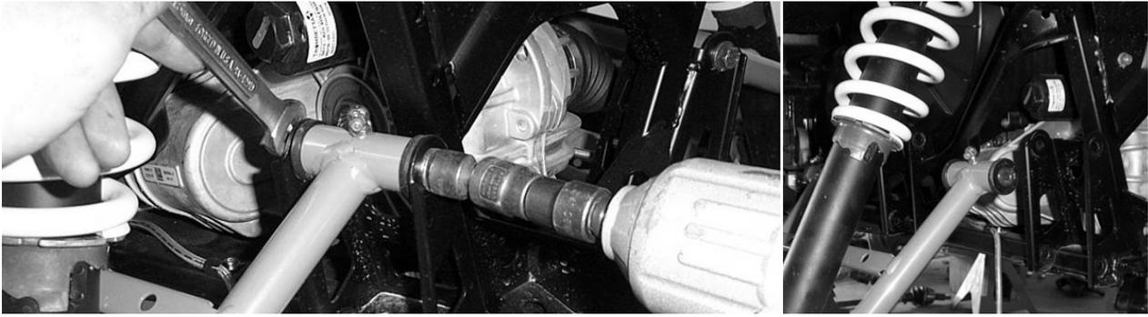
12. At this time, it will be easier for you to extend the brake lines. Included in the kit are two 6" brake line extensions for the rear.
