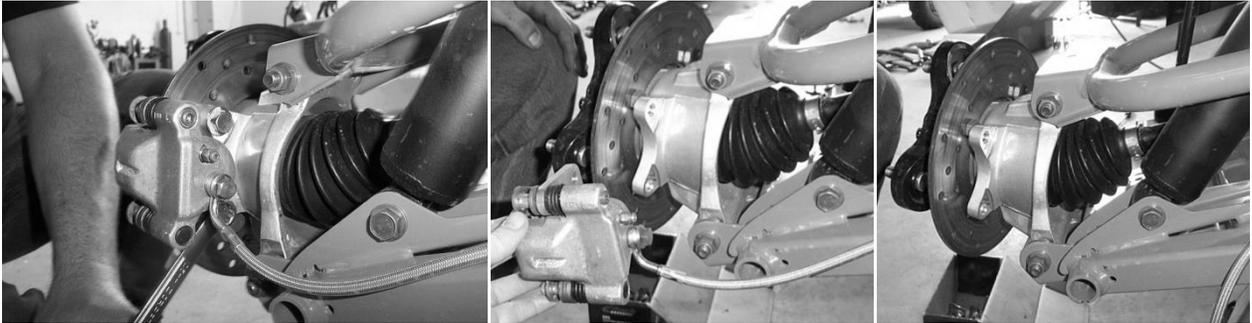
4. Disconnect and remove the factory cotter pin and castle on the rear axles.
