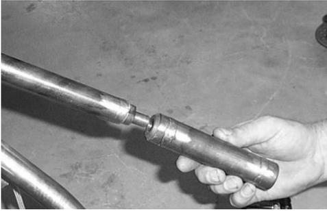
51. You will need to use a 1/2" drill bit to drill out the factory hole with the original tie rod connected.
