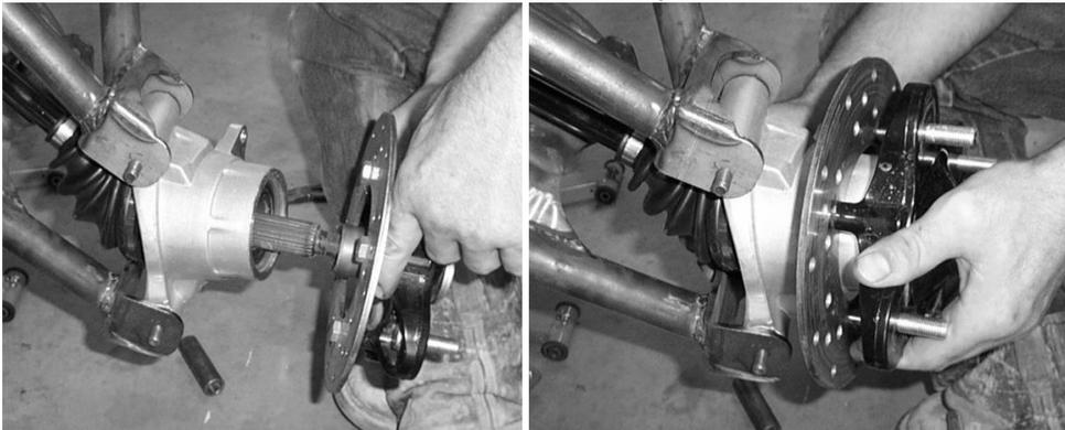
32. Fasten the rotor using the axle washer, castle nut, and cotter pin provided in the kit.
