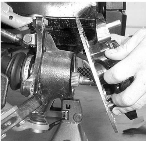
6. Disconnect the upper and lower arms and tie rods from the front hub assembly.
