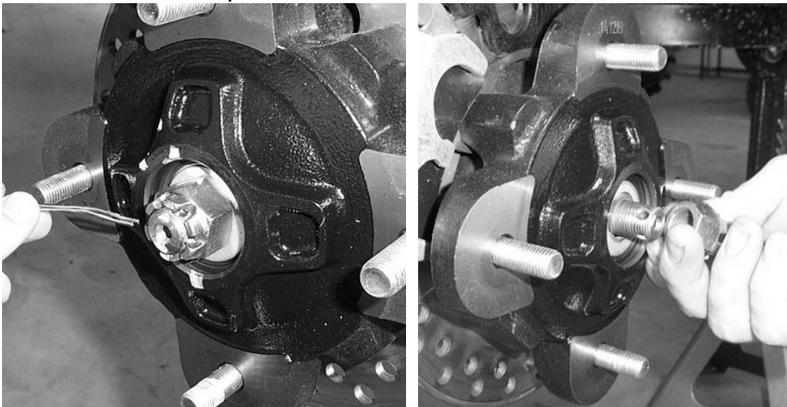
5. Remove the brake rotor.
