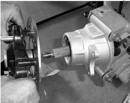
6. Disconnect the upper and lower control arms from the hub assembly and remove the hub assembly.
