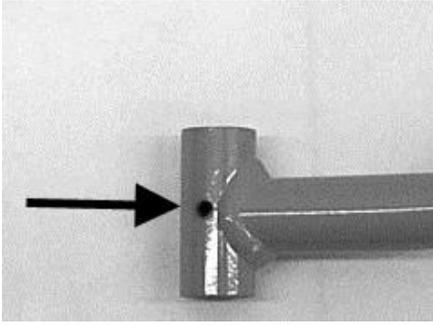
19. Once you have removed the stock bushings and sleeves from the factory arms install them into the new arms in the kit. If you place some grease on them it makes the installations easier.
