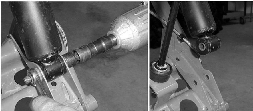
11. Remove the upper and lower rear control arms from the UTV. You will reuse the factory hardware to reconnect the new control arms to the frame.
