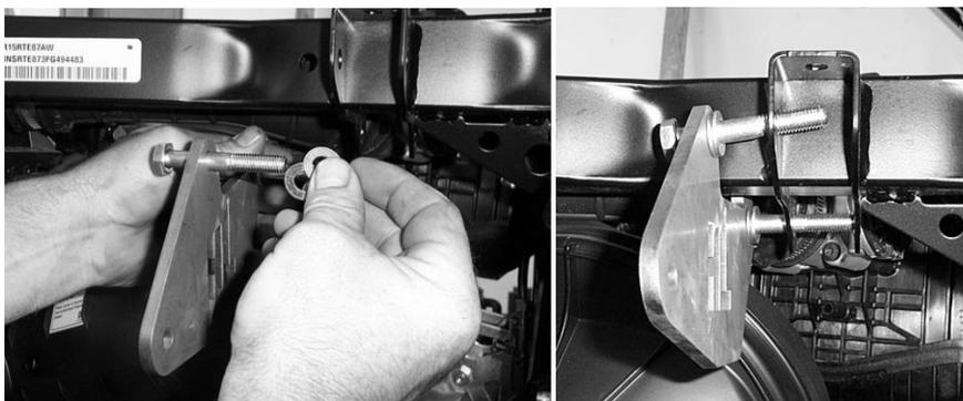
36. Now insert a spacer on each of the bolts and the other rear lift bracket to the inside of the shock mount tab. Loosely fasten it with two 10mm lock nuts.
