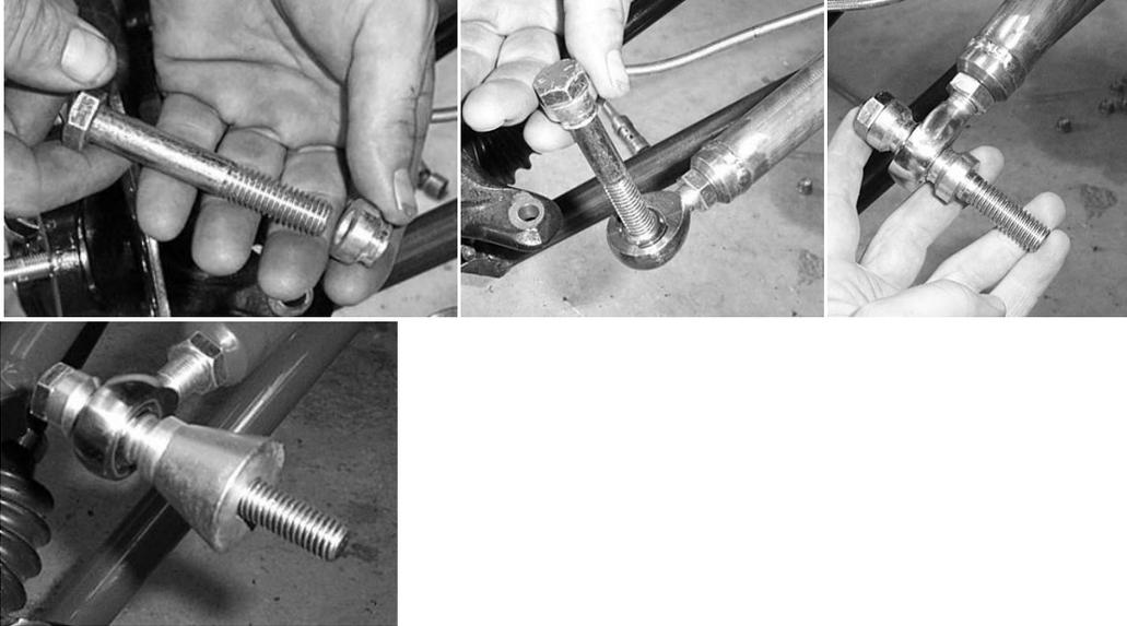
55. Insert the new  $\frac{1}{2}$ " x 4-1/2" hex bolt. Slide the bolt through the alignment bushing, large cone then the heim joint and then through another alignment bushing. Insert the bolt through the knuckle assembly.
