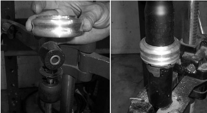
21. Place spring back on the shock, compress it, and then reinstall the retaining clip.
