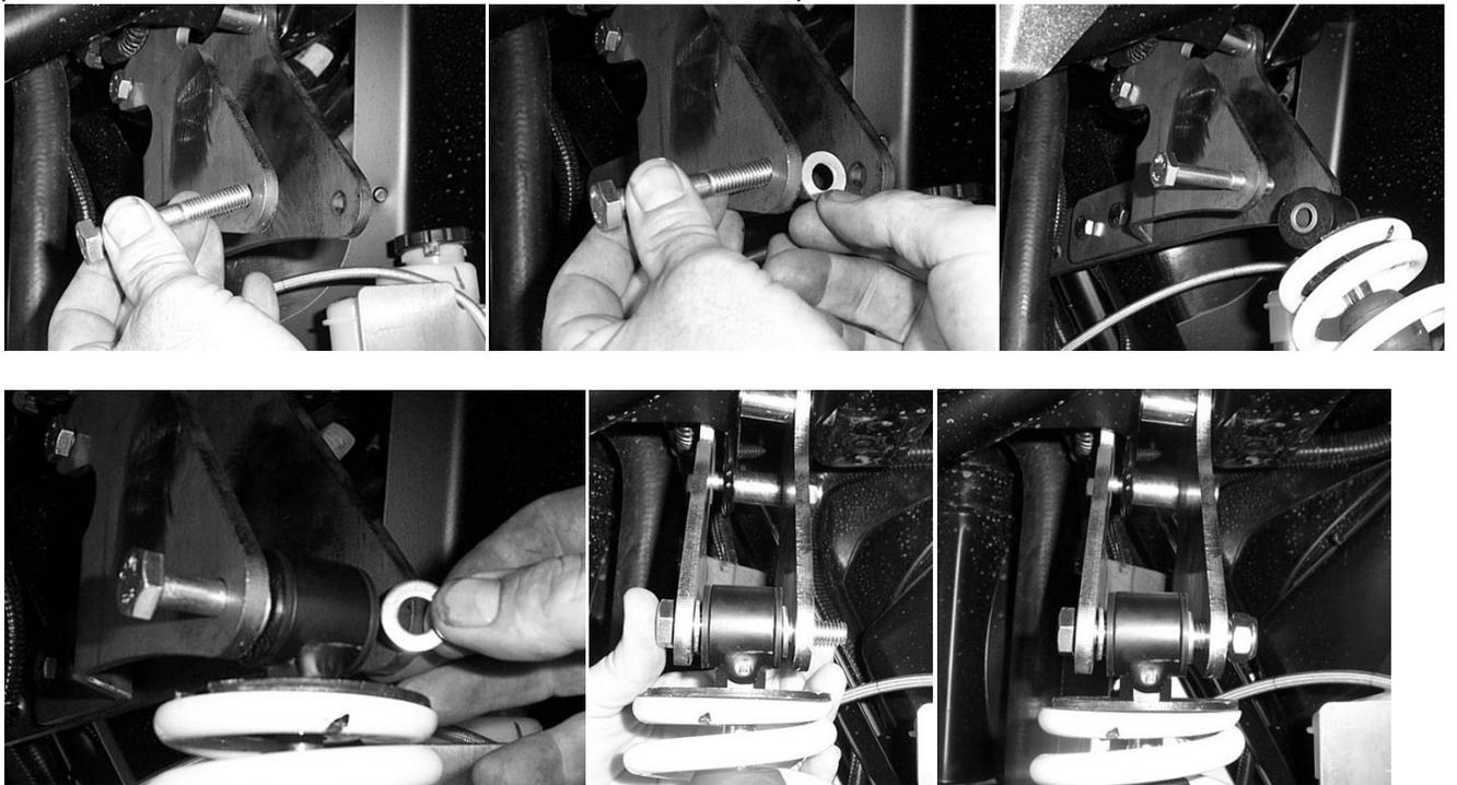
47. Connect the lower portion of the shock to the new control arm using the factory hardware.
