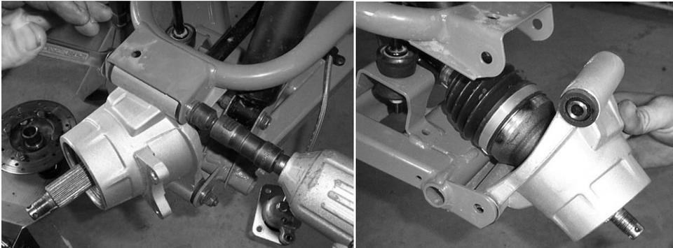
7. Pull the axles out of the differential.
