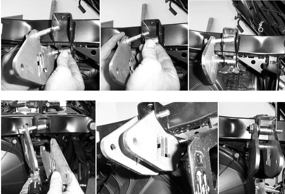
37. Connect the top of the shock to the lift brackets using one 10x65mm hex bolt and 10mm lock nut.
