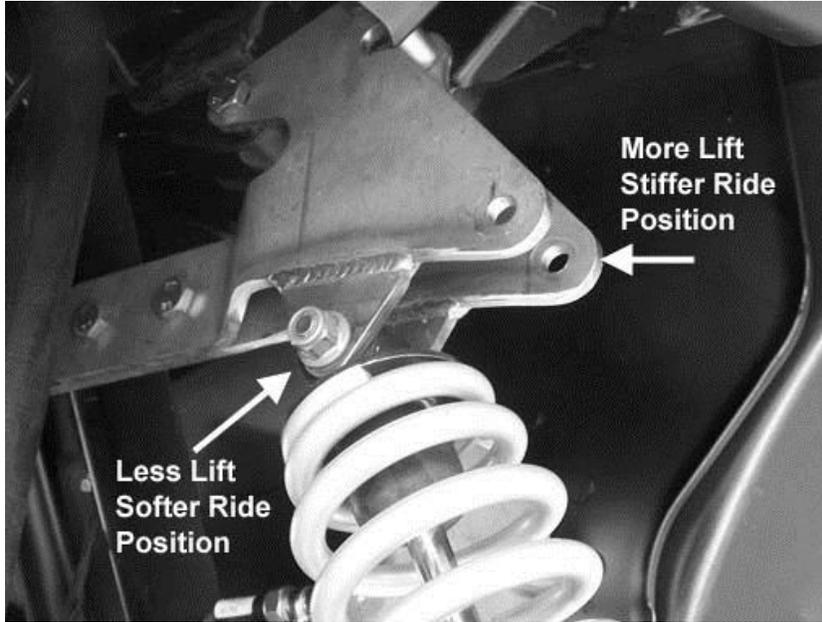
46. Now connect the upper portion of the shock to the lift brackets with the 10mm x 65mm bolt and 10mm lock nut provided. Place a 10mm washer in wither side of the shock eyelet, between the brackets.
