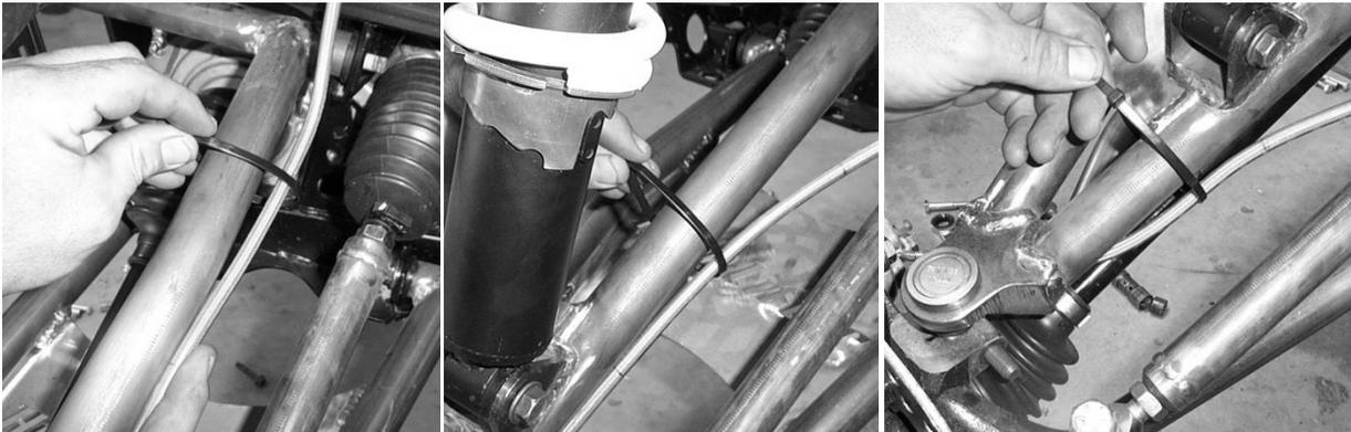
49. Slid the new tie rod sleeve over the factory tie rod, screwing into place.
