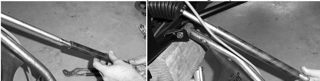
50. Next connect the smaller tie rod extension to the end of factory rod.
