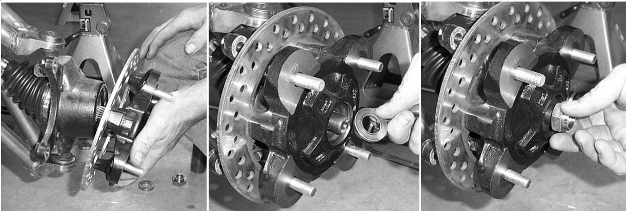
44. You must use a punch to secure the axle nut in place on the axle end when the axle nut is tight. If you do not use a punch to secure it in place it will back off the axle.
