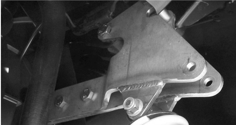
34. Insert the bolts from the front to the back and fasten them with the 10mm lock nuts provided.
