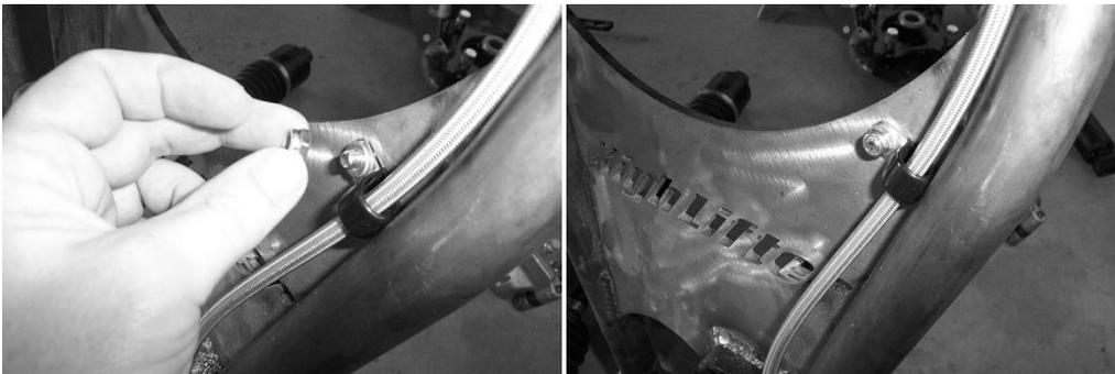
43. Uses zip ties provided to secure brake line.
