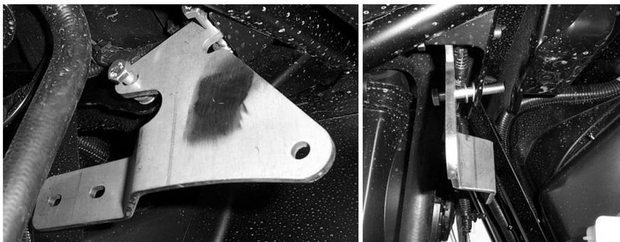
32. Now insert a spacer on each of the bolts and the other front long lift bracket to the inside of the shock mount tab. Loosely fasten it with two 10mm lock nuts.
