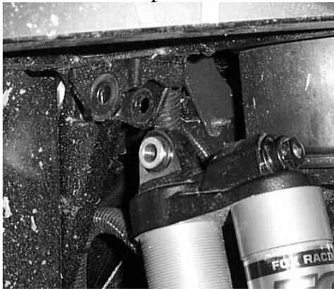
8. Rotate the piggyback reservoir on the shock 180 degrees. Rotates very easy by hand.
