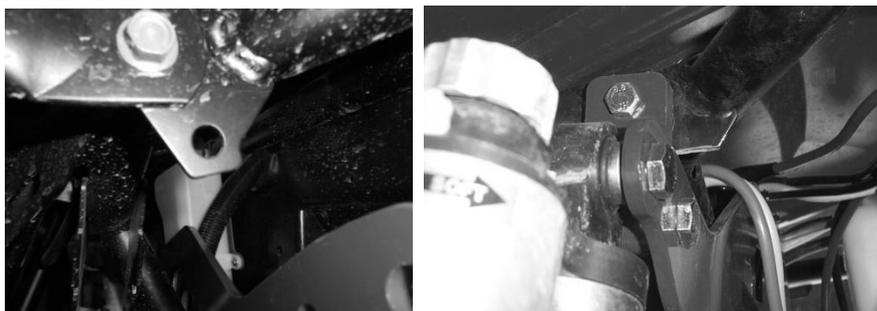
9. Connect the top of the shock to the lift plates, using the outside holes, by placing 10mm flat washers on either sides of the shock eyelet and securing using the 10 x 65mm hex bolt and 10mm lock nut.
