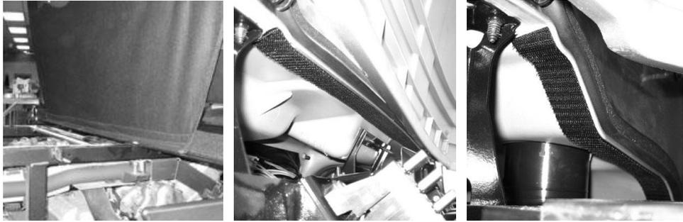
6. Now loosely drape the Cab Enclosure over the Ranger Crew roll cage. While having someone holding the hood up or propping it up, slip the middle nosepiece between the hood and dash and attach it to the adhesive Velcro underneath the dash. Next pull the side nosepieces under the dash and attach to Velcro there. Finished look should be like photos below.
