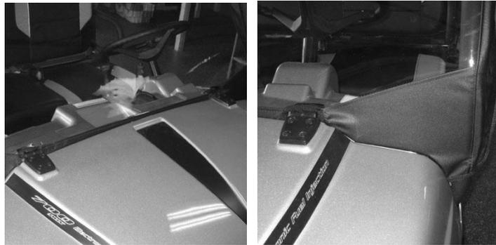
7. Now note the positions for the two 10" tabs on either side of the windshield. Attach the coordinating adhesive strips to the inside of the roll cage.
