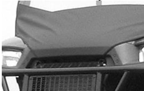
6. Next raise the bed and place the 40" adhesive Velcro strip across the bottom rear of the cab, centered on the metal strip. Now pull down on the rear of the cab enclosure and affix to the Velcro. See Photo at top of next page:
