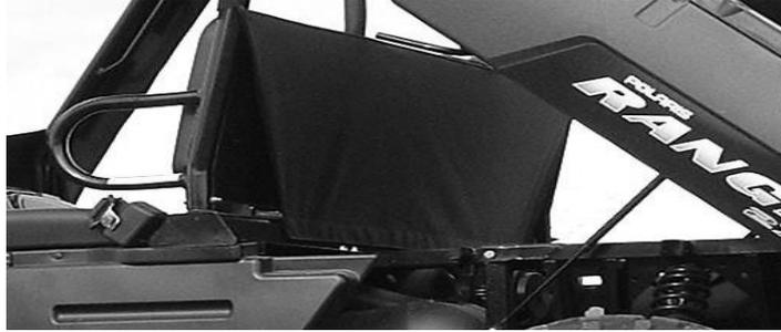
7. Next place the two 10” adhesive Velcro strips on both sides of the rear window to match up with the corresponding tabs.
