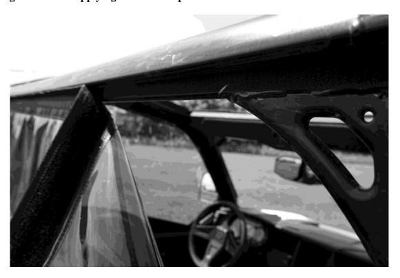
3. After the adhesive Velcro strips have been installed along the top and down the sides you can now place your rear window in the frame. Lastly mark where the bottom of the rear window sits on the vehicle and place the 48" adhesive strip flat on the vehicle so the bottom of the rear window pulls into the cab and attaches downwards.
