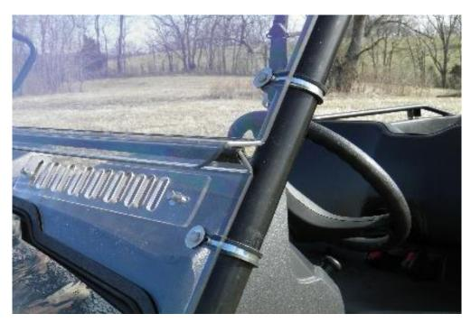
**Step 8:** When satisfied that the upper windshield section is positioned properly, tighten the knob bolts. Attach nuts to the knob bolts to hold in place.
