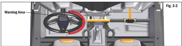
Check all positions of the steering column making sure that you have clearance for your hand to operate the vehicle in all positions.
