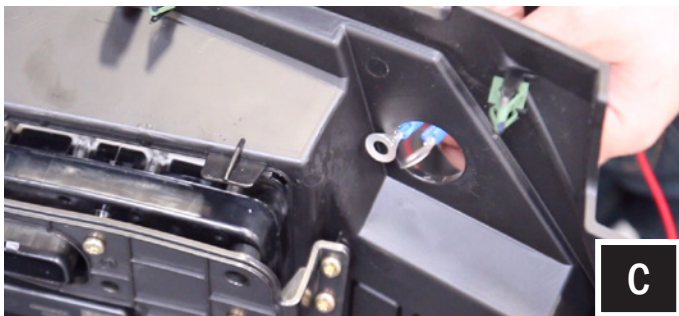
C. Feed in the wires and cable through the factory 12v hole. Keep the fuse holder open and empty until it has passed through the hole.
