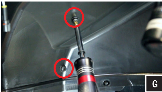
G. With the provided M6 screws and washers, loosely mount the pod through the 3 holes previously drilled. Once all screws have been inserted into the pod, hand tighten all 3 screws.
