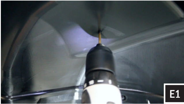
E. Drill a pilot hole at the places just marked with a 1/8" drill bit. Then follow up by using a 1/4" drill bit for both pilot holes (for mounting the pod).
