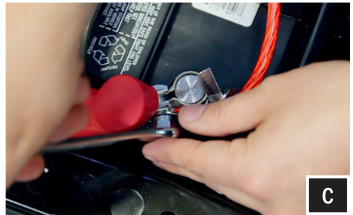
C. Unscrew the factory nut on the positive battery terminal. Install the 2 power cables to the screw on the positive battery terminal. Re-install the factory nut.
