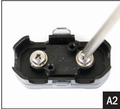
A2. Extract both fuse holder screws.
