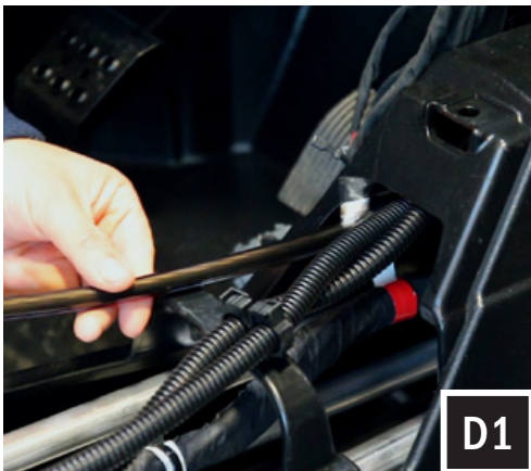
D. Feed the connector end of the Amp power wire through the center console to the other side of the firewall (D1). Then feed the power wire through the grommet hole (D2) and through the rubber grommet with the rest of the vehicle's wiring and cables (D3). Do the same for the 2nd Amp power & rear speaker wire.
