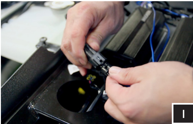
I. Route the speaker wire away from any moving parts and any sharp metal, then connect to the amplifier.
