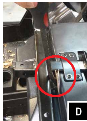
D. To properly align the box, slide the box firmly toward the front of the vehicle. It should sit approximately 1/4" from the factory glove box mount. If not properly installed, the kick pod and dash panel will not align in place.
