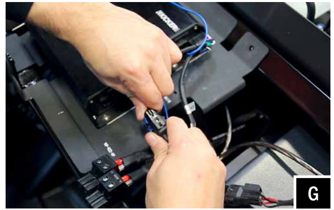
G. Connect the B-H1151 speaker harness to the amplifier
