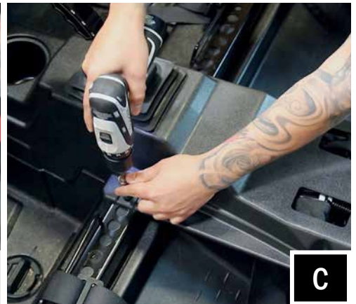
C. Remove all of the center console push pins and T-30 Torx screws. For 4-seat models, disconnect the harness attached to the 12v accessory socket.
