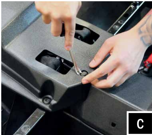
C. Remove all of the center console push pins and T-30 Torx screws. For 4-seat models, disconnect the harness attached to the 12v accessory socket.
