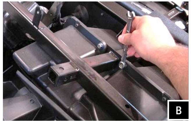
B. Remove the two 10mm bolts that secure factory glove box and remove the factory glove box
