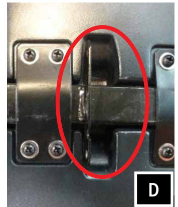
D. To properly align the box, slide the box firmly toward the front of the vehicle. It should sit approximately 1/4" from the factory glove box mount. If not properly installed, the kick pod and dash panel will not align in place.
