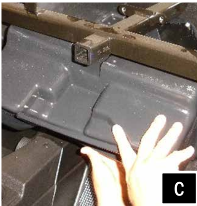
C. Lift the enclosure into place and align the top channel in the grab handle bar. While holding the enclosure in place, loosely attached the flat brackets to the top of the enclosure using the long screws provided.
