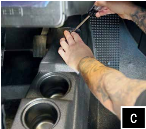
C. Remove all of the center console push pins and T-30 Torx screws. For 4-seat models, disconnect the harness attached to the 12v accessory socket.
