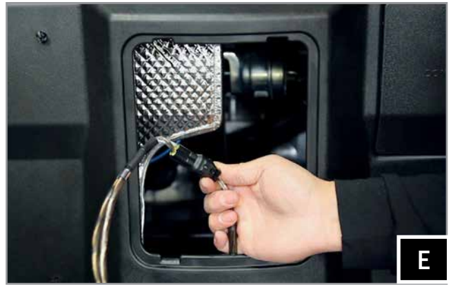
E. From the rear of the center console, route the B-H1150 harness up to each speaker pod and connect.
