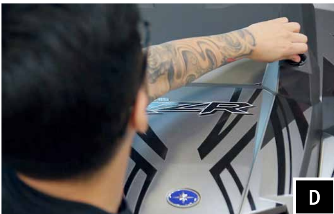
D. Remove hood by turning locking pins and lifting up.
