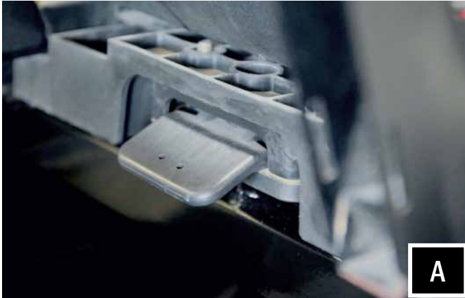
A. Remove driver seat by releasing the handle behind each seat, push forward slightly while lifting up
