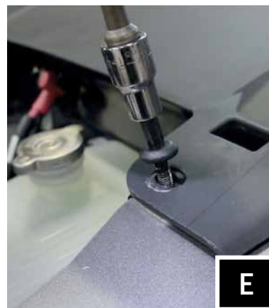
E. Remove center dash by unscrewing the 2 T-30 Torx screws and push center dash forward to unclip.
