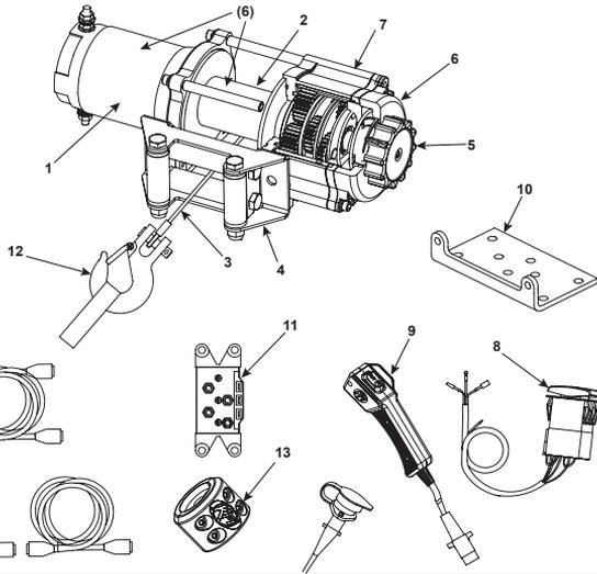
**Motor (1):** 1.7 HP 12V DC motor provides power to the planetary gear mechanism.
