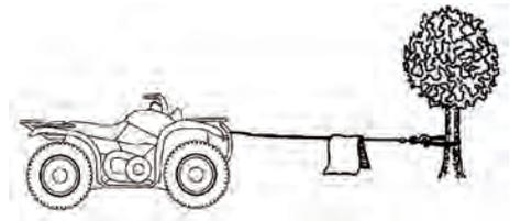
In the event of a broken cable it will dampen the snap back. For additional protection open the hood of the vehicle.
