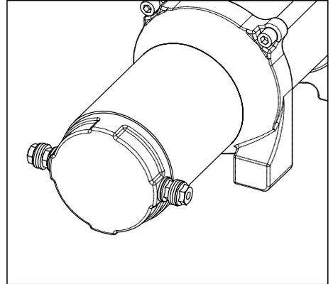
With some applications the motor leads may need to be rotated to avoid interference with other components. If rotation is required please give us a call at 1-877-346-2050 for instructions or visit our website at [www.kfiproducts.com](http://www.kfiproducts.com) and look in the Instructions section.
