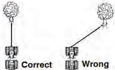
Short pulls from an angle can be used to straighten the vehicle. Long pulls should be done with the wire rope at a 90° angle to the winch/vehicle.
