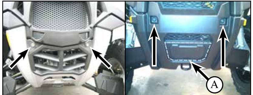
"Figure 2" Removal of Front Plastic
