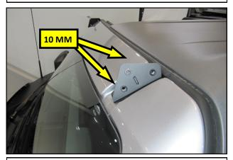
**4.** Install the Light Bar Brackets onto the vehicle a shown, using the OEM nuts removed in step **2**. Leave the nuts sung at this time.
