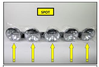
**5.** Mount the lighting to the RTR Base. Lighting can be mounted to the face of the Base or on top of the Base. **NOTE:** Verify that the intended light mounting method will not interfere with the vehicle once installed.
