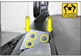
**6.** With the help of an assistant, lower the Light Bar assembly onto the Light Bar Brackets. Secure the Bar on each side using the 6mm Button Head Bolts. Leave the bolts snug for now.
