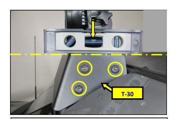
**8.** With the vehicle parked on level ground, place a level on the top of the Light Bar as shown. Adjust the angle of the Light Bar as needed to get it parallel to the ground. Tighten all six light Bar screws, final tight.
