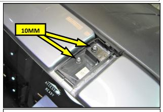
**2.** Using a 10 mm socket, remove the flange nuts securing the cap retainers to the vehicle. Retain the nuts for reuse.
