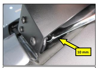
**7.** Using a 10mm wrench, tighten the 4 Bracket nuts from steps **29** and **30**.
