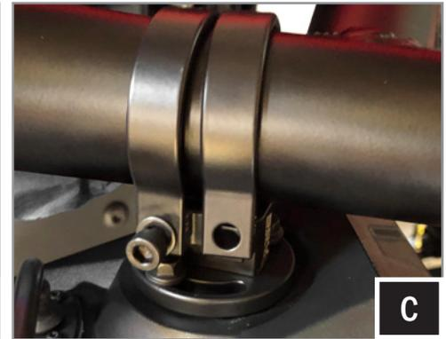
C. Wrap a plastic bag around the roll cage to prevent scratching. Press the clamps onto the roll cage over the plastic bag. Place the (2) M6x1.0x45mm screws and washers through the clamp and clamp base. Secure the clamps to the roll cage with a 5mm allen key.
