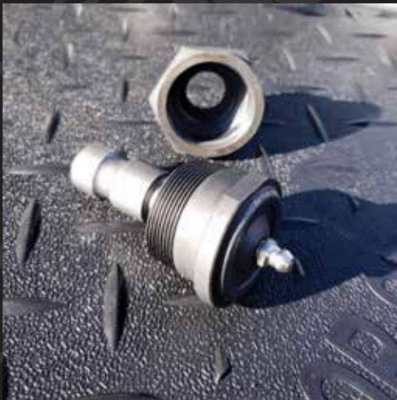
1. Remove dust boot from ball joint.
