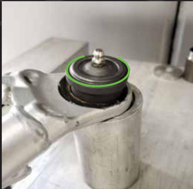
2. Press ball joint into arm until seated properly. Apply force only on the HIGHLIGHTED AREA.
