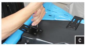
C. Once the enclosure is centered side to side, press the bracket toward the center of the vehicle and tighten the brackets using the #3 screwdriver.
