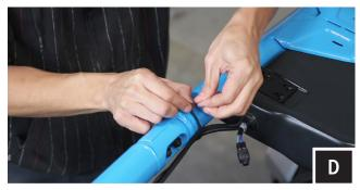
D. Using the zip ties provided, route the Power/Ground loom to the battery location away from any moving parts or sharp metal. NOTE: The 4 pin short cable is for additional speakers and the 4 pin long cable is for adding an SSV Works Powered Subwoofer (Part# WP-CMS10)
