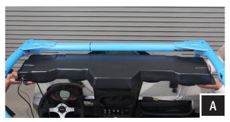
A. With one person on either side of the vehicle place the WP3-CM04A into location from the underside of the cage.
