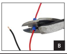
B. Crimp the supplied fuse holder onto the end of the RED wire and attach to the battery "+" terminal.
