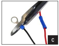
C. Crimp the supplied ring terminal to the BLACK wire and attach to the battery "-" terminal.
