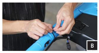
B. While holding the enclosure securely toward the front crossbar of the cage, loosely install the 4 brackets using the screws provided.
