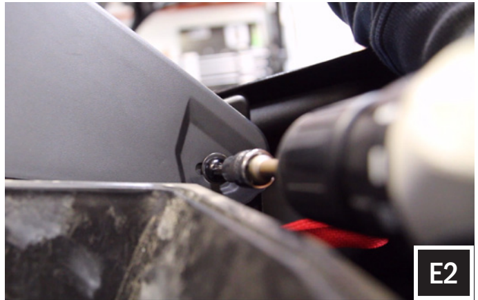
E2. Using panel removal tool unsnap (2) push clips on the driver and passenger side dash covers. Unscrew the (4) T30 screws on the passenger side, and (7) T30 screws on the driver side.
