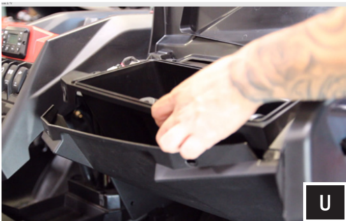
U. Pull up and remove the glove box.
