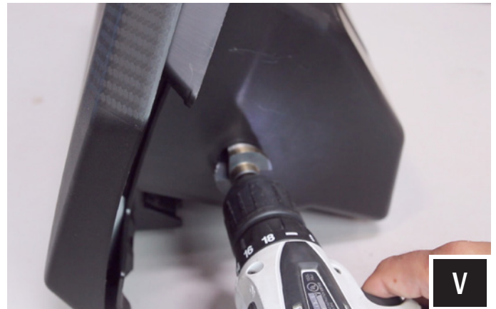
V. Drill a 1" hole through the left side of the glove box for wiring
