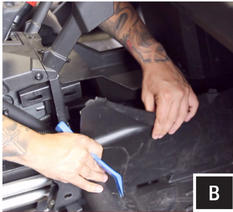
B. Carefully unsnap center console panels by hand or with a panel removal tool.
