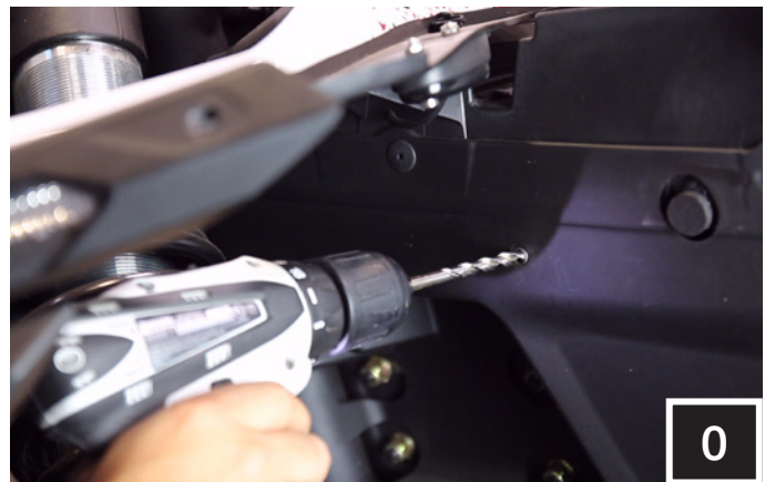
O. Drill a larger hole through the pilot hole using a 1/4" drill bit. Be sure to move the amp plate out of the way before drilling.
