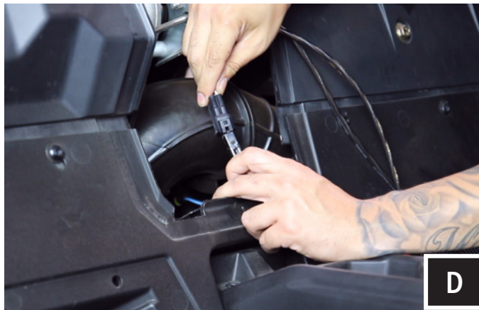
D. Take the B-H1150 rear speaker harness and plug into the B-H1151 rear extension harness.
