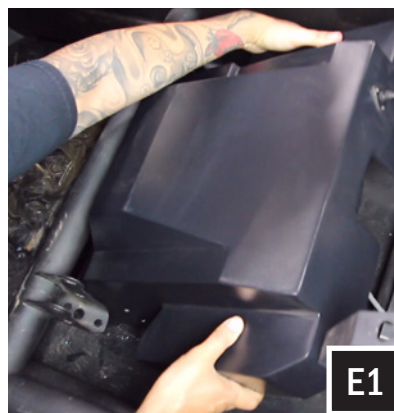
E. Run the brake line along the dedicated channel on the sub enclosure while feeding the enclosure down under the seat bar (F1). Make any adjustments to the brake line so the enclosure lays on top of it. Line up the rear enclosure brackets to the rear seat bolts and press down until the brackets rest on top of the spacers.
