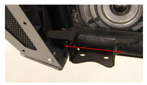
8.) INSTALL TOP HALF OF BUMPER TO BASE. IF RIGID ARM OPTION WAS PURCHASED, INSTALL TAB BAR ON TO TOP HALF TABS (2) 3/8-16 X 1" BHCS), AND CONNECT RIGID ARM TO LIGHT BAR (2) 3/8-16 X 1.5" BHCS).
