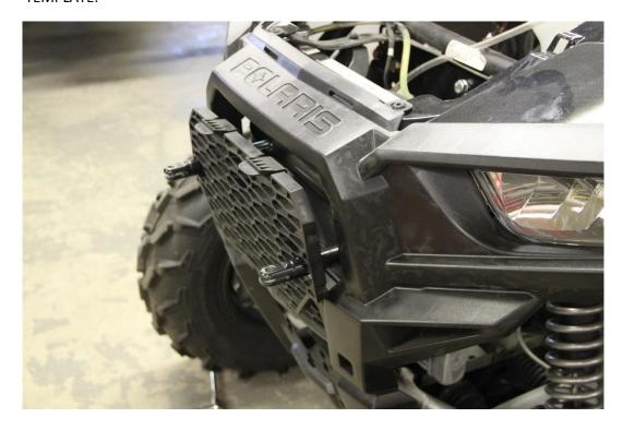
5.) ASSEMBLE FRONT BASE SECTION OF BUMPER. DO NOT INSTALL TOP PLATE BOLTS UNTIL YOU INSTALL THE TOP SECTION OF THE BUMPER.
