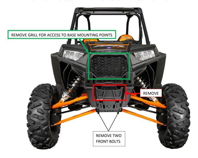
2.) TEAR DOWN NEEDED TO INSTALL THE BUMPER WITH RIGID MOUNTS: FIRST JACK UP YOUR RZR, SECURE WITH JACK STANDS, THEN REMOVE THE FRONT LOWER A-ARM BOLTS (JUST THE FRONT TWO BOLTS), GRILL, AND FRONT FASCIA. YOU WILL NEED TO UNHOOK THE HEADLIGHT CONNECTIONS TEMPORARILY.
