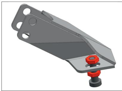
7. Fix door lock axle no.4 on bracket no.3 using thin (low) nuts no.16
