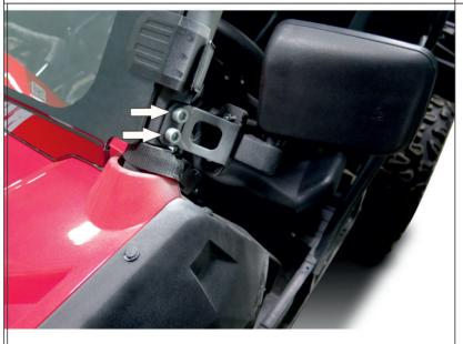
6. Remove the screws M10 which are fastening the cage elements in the front side.
