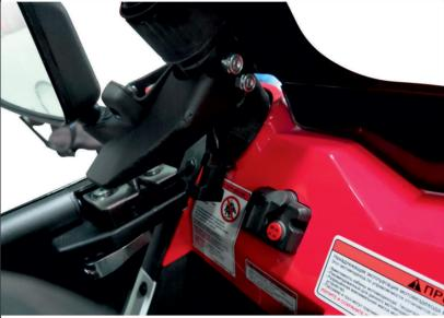
8. From the inside, install spacers no.5 into the slots of the cage. Fix door lock bracket no.3 together with original rear view mirror using screws no.12, washers no.20 and nuts no.15.
