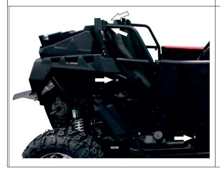
9. Fix base door assembly no.1 to the original fastening points of the side tube: using screws no.10 and washers no.18 for the upper points, using original fasteners for the middle and lower points.
