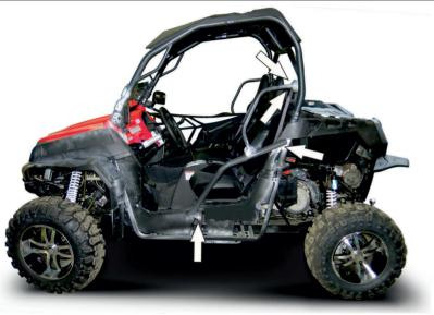
5. Remove the screws indicated by the arrows. Remove the original cage tubes.
