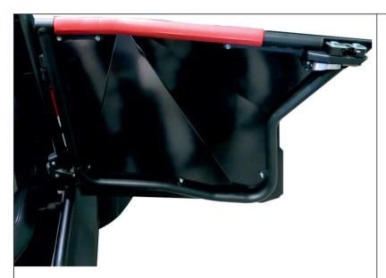
10. Mount doors no.2 on the hinges of base no.1. Fix opening limiter no.23 on doors no.2 using screw no.9, washers no.17 and nut no.13.
