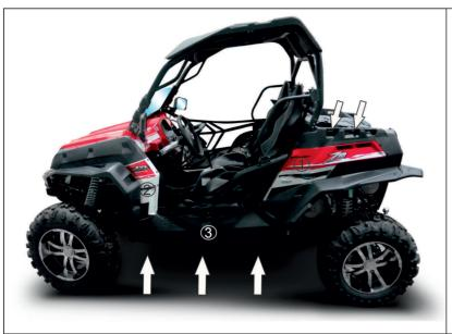
4. Turn off the screws indicated by the arrows. Remove all the pistons from plastic covers 1, 2, 3. Remove panels 1, 2. Remove two bolts M6 which are hidden by panels 1, 2 and then remove the pistons. Remove panel 3.
